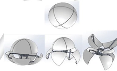
Fig. 9. BALL-E Robot with spherical & quadruped configurations
