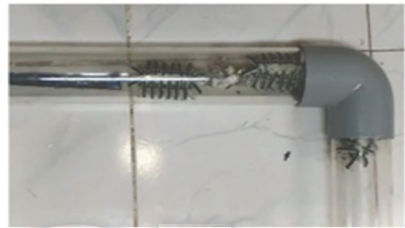
Figure 4: Pipe climbing robot passing through a 90° bend pipe.
